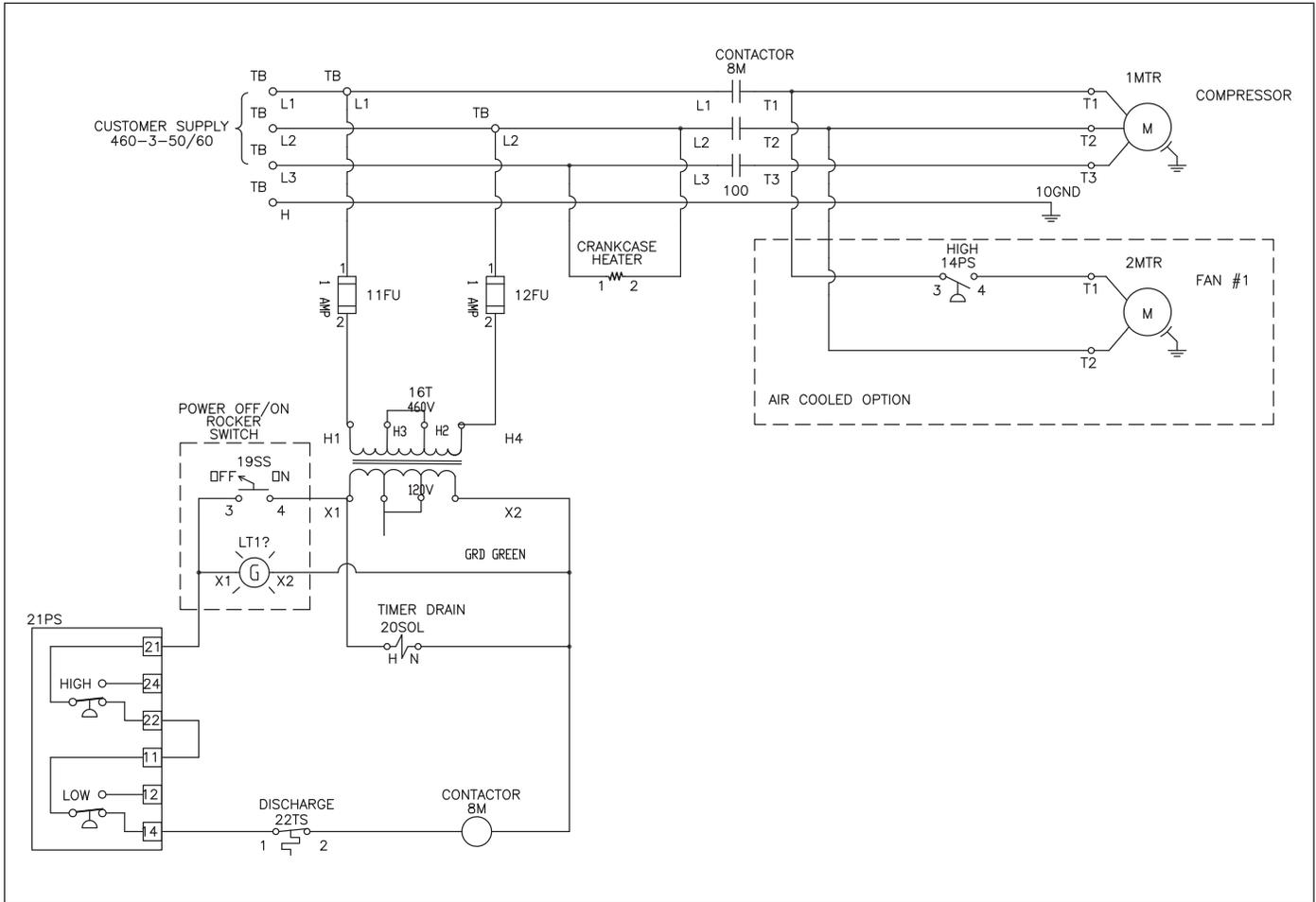
Wiring Diagram, 2-5 HP Models: 3 Phase, 460 Volt, 60 Hz
