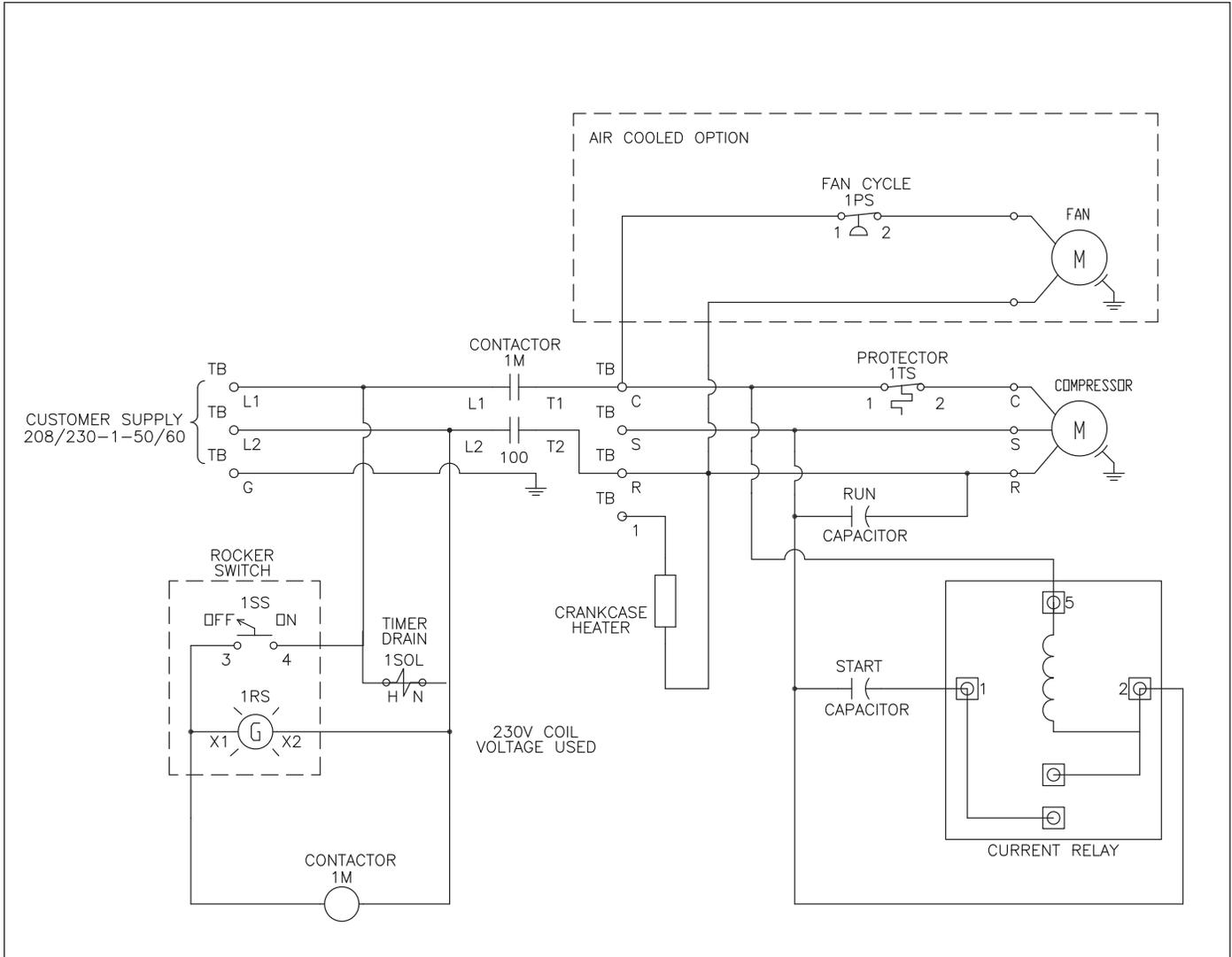
Wiring Diagram, 1-1/2 HP Models: 3 Phase, 230 Volt, 60 Hz
