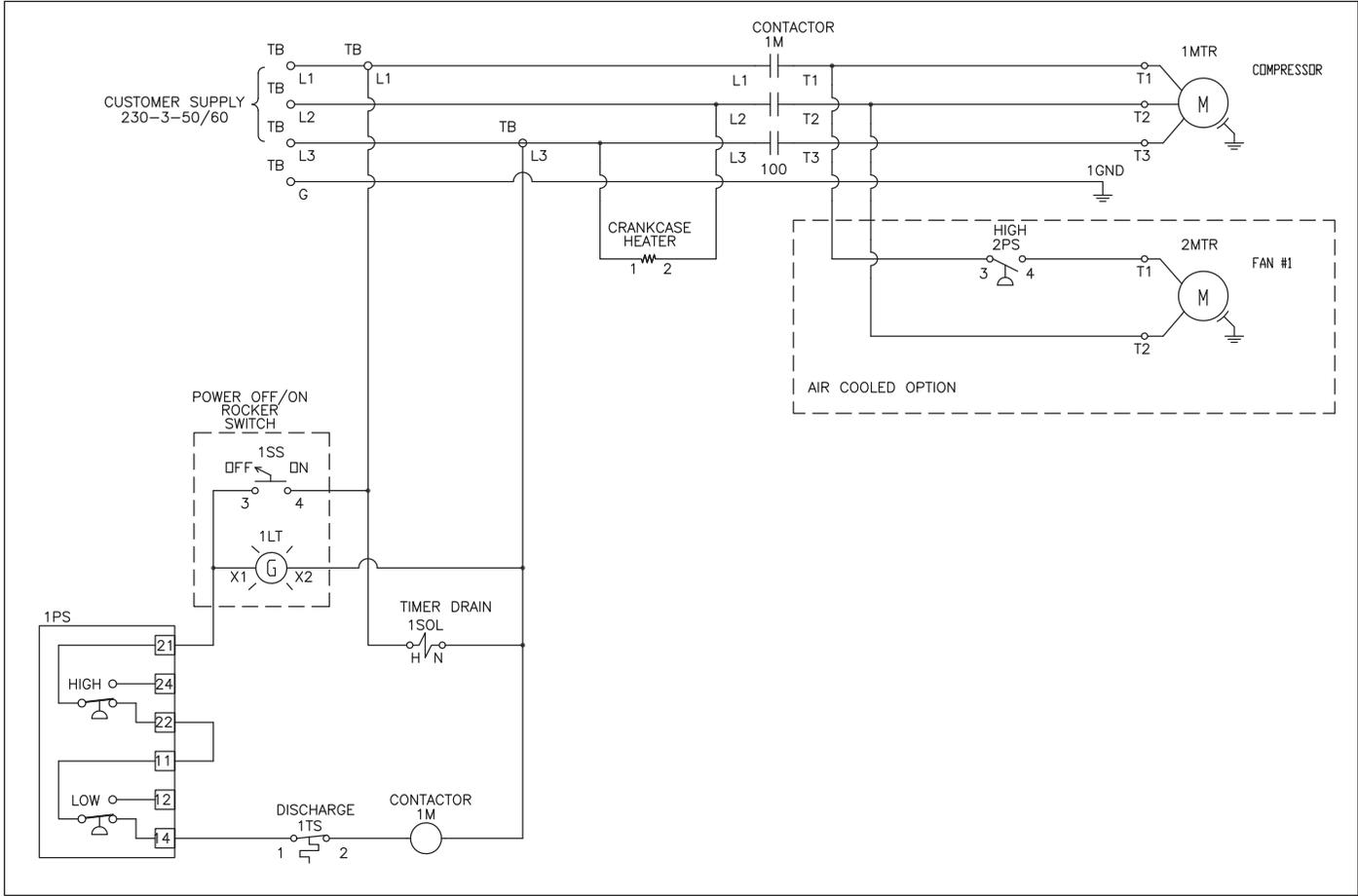
Wiring Diagram, 1-1/2: 3 Phase, 460 Volt, 60 Hz
