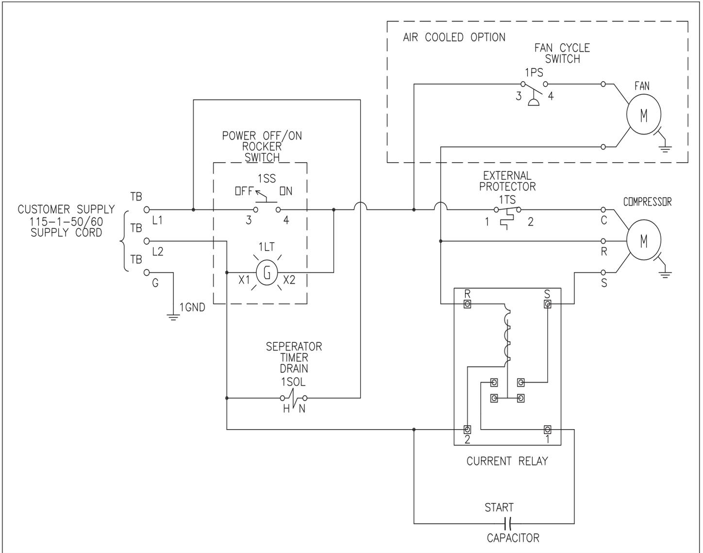
Wiring Diagram, 1/2 - 3/4 HP Models 1 Phase, 120 Volt, 60 Hz
