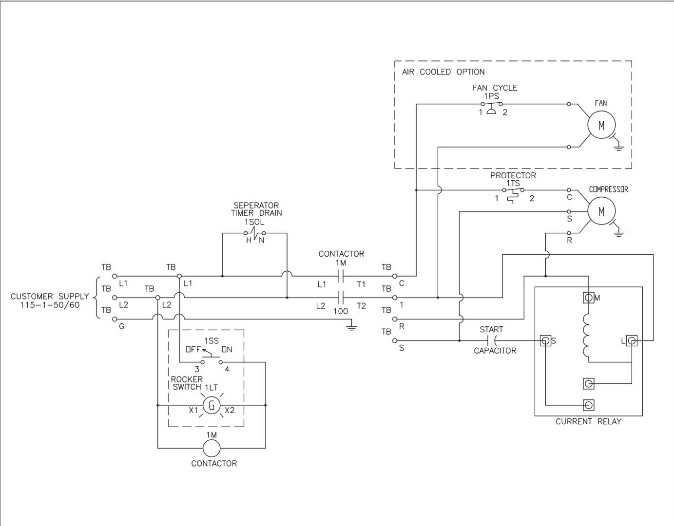
**Wiring Diagram, 1-1/4 HP Models: 1 Phase, 208/230 Volt, 60 Hz**
