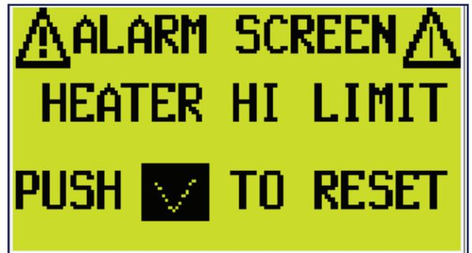
FIGURE 5-28: Heater High Limit
