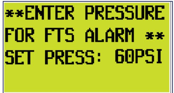
FIGURE 5-2: Failure To Shift Entry Screen
