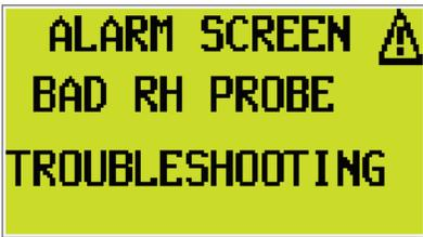
**Bad RH Probe:** Shows when the relative humidity (EMS) probe is out of range. This can be either high out of range or low out of range. When this happens, the signal has either been lost or the sensor may need to be replaced.
