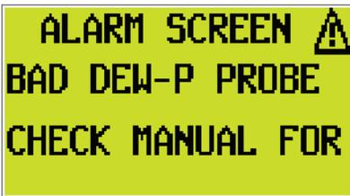
**Bad Dew-P Probe:** Alarm for the dew point sensor probe out of range. The out of range can be either high or low. This can be either a complete loss of signal/voltage, the resistor can be disconnected or the sensor may need to be calibrated.
