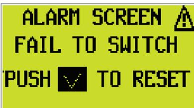
**The FTS Alarm (Failure-to-Shift):** Alarm present when a vessel does not depressurize correctly or if a vessel that is to be drying does not have pressure at or above a certain set pressure.
