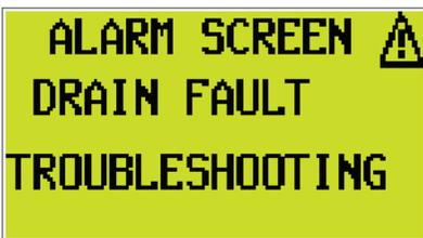
**Drain Fault:** Shows when the relative humidity (EMS) probe is out of range. This can be either high out of range or low out of range. When this happens, the signal has either been lost or the sensor may need to be replaced.
