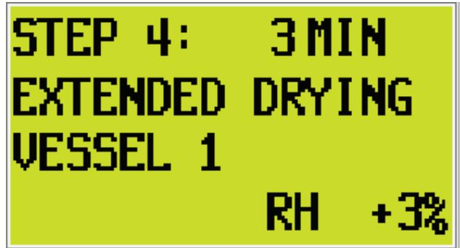
**Note:** If the dryer needs to continue to the next step to regenerate based on humidity, the extended savings step 4 will be skipped.
