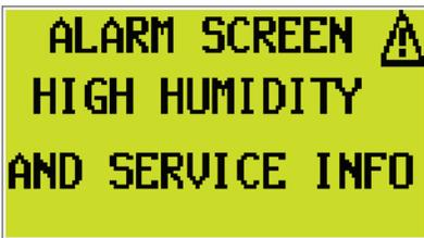
**High Humidity Alarm:** Alarm that is visible when the dew point is higher than the set point. The set point for the high humidity alarm can be changed but it is not recommended.
