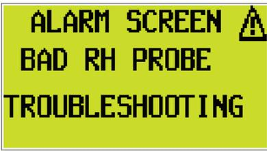
**Bad RH Probe:** Shows when the relative humidity (EMS) probe is out of range. This can be either high out of range or low out of range. When this happens, the signal has either been lost or the sensor may need to be replaced.
